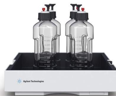
InfinityLab solvent cabinet, with solvent bottles and Stay Safe caps
